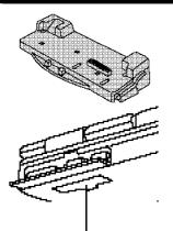
The port replicator (CF-VEB251) connects to the expansion bus connector on the bottom of your computer.
